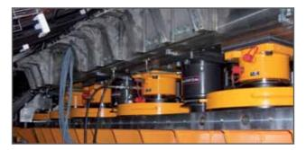
Load tests made on a cut off wall in the bearing structure of a buildings foundations.
