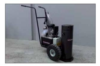
High tonnage cylinders with retractable wheels to make handling easier. They are oil return cylinders, equipped with safety nut, integrated tilt saddle, gauge and pilot check valve to operate safely.
