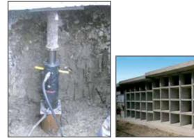
Strengthening of a motorway viaduct with a test on a 1000 mm diameter cement pile with an induced load of about 700 ton. (Italy, Piacenza 2008)
